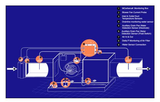
This schematic illustrates the typical installation for a Roof Top Unit
