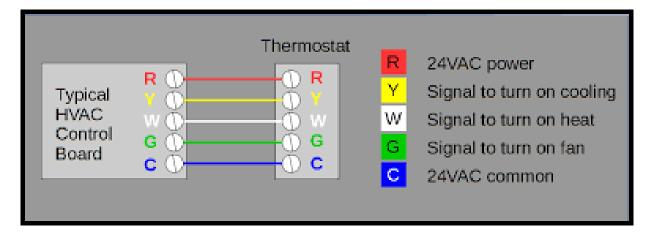
A power connection is integrated into the MCerberus® monitoring box. Each of the wires is identified by the following schematic.
